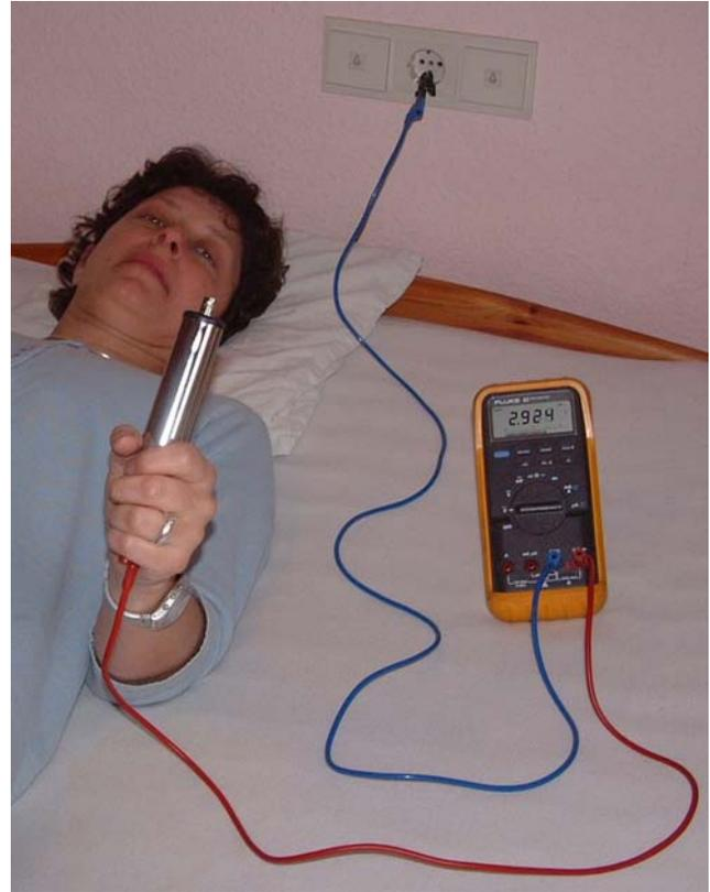
**Figure 1: Body voltage testing against ground potential with a digital multimeter**
