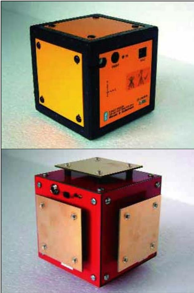
**Figure 2: Potential-free, 3-D E-field probes, also referred to as “cube sensors” due to their shape; in order not to have a metal cable interfere with the electric field, the connection to the data analysis and display unit is provided by a several-meter long fiber-optic cable, thus ensuring correct measurements of the electric field in any situation**
